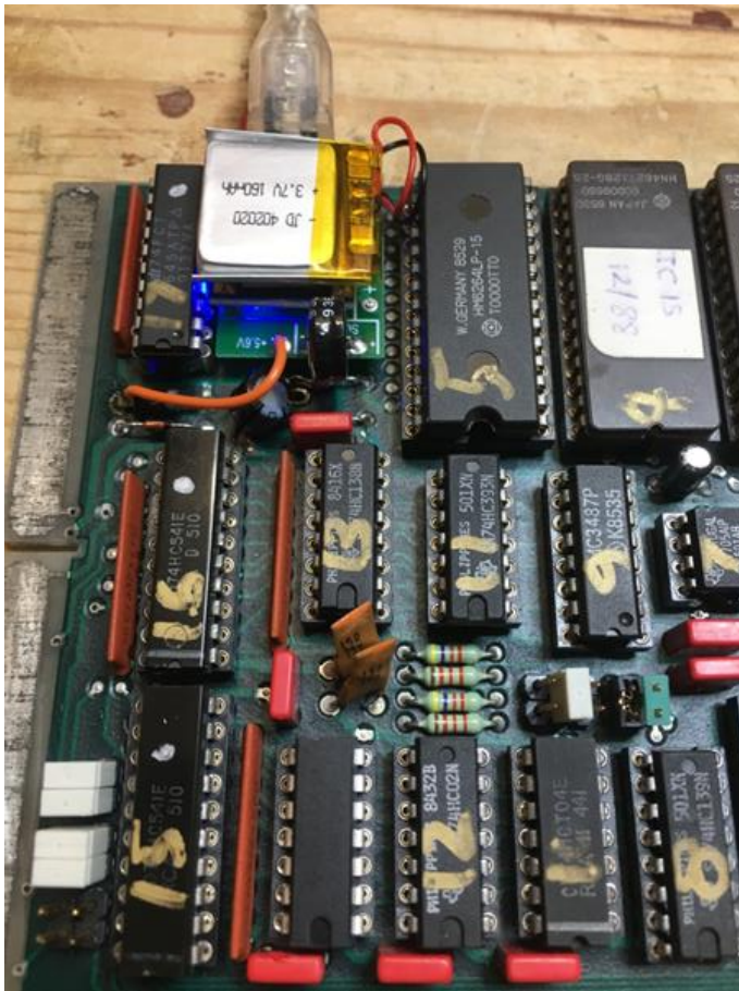
Above. Studer A812 Backup battery installation.
